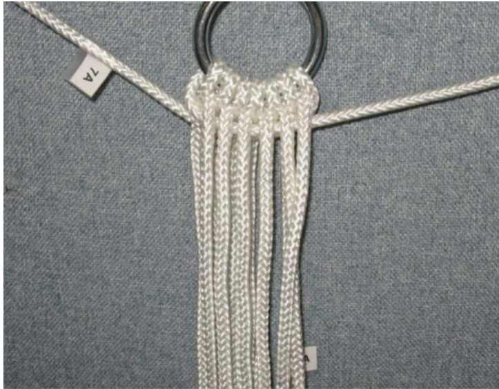
Figure 4 Passing the Strands Steps 5 and 6
